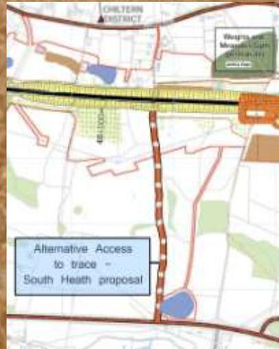
**Proposed road to access the trace between South Heath and the Wendover viaduct. The new road follows footpath GMI/12/1, but could join the A413 at the "Link Road" roundabout, if this reduced congestion.**
